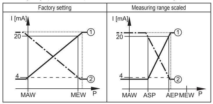
P = system pressure , MAW = initial value of the measuring range, MEW = final value of the measuring range
